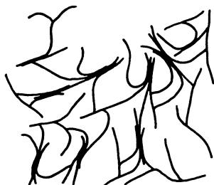
Figure 8. Micellar Organization Within Swollen Starch Granule, According to K. H. Meyer Micellar regions indicated by thickened sections
